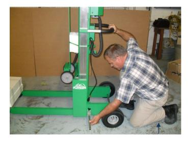
Tighten the triangular screws on each side of the LIFT. **Be sure to tighten BOTH sides**.
