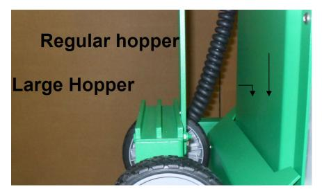
The **inside** channel (closest to the LIFT) is for a **regular hopper** machine; the **outside** channel is for a **large hopper** machine.
